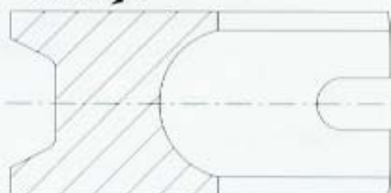
Raschiaolio Oil scraper ring Mark
