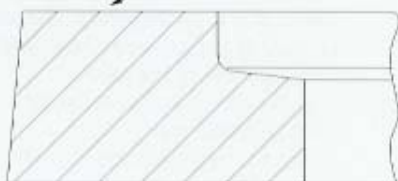
2° segmento 2nd piston ring Mark
