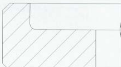
1° segmento 1st piston ring
